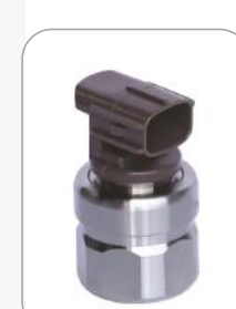
BG NO.: DENSO - L:145uh FOR INJECTOR: 0950005600/6240/6241/624/6243 0950005760/6791/6521/5650/5655 0950006251/6252/6253/6790/6250 1465A041
